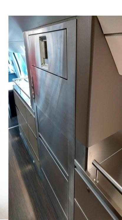
The material lift enables the transport of a minibar to the upper floor of a double-decker rail vehicle. This enables the passenger to consume from his seat in comfort. The material lift is limited to 180kg payload. A special feature is the continuous cabin. This makes it possible to reach even the middle deck.
